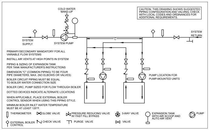
Figure 7. Hydronic Piping — Primary-Secondary, Reverse-Return.
